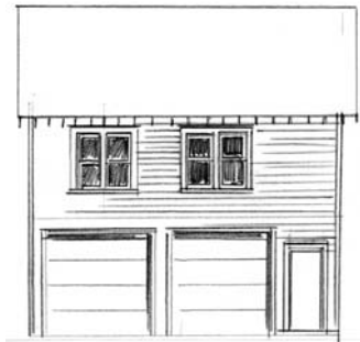
Elevation of a Garage Apartment
