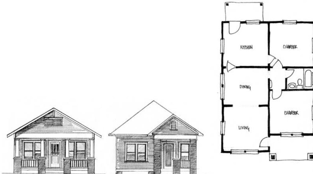
Elevation of 2106 Decatur Elevation of 606 Hemphill Typical Floor Plan of a Bungalow
